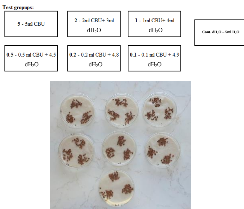
Figure 17: Experiment design of flaxseeds germination test, assessing the toxicological aspect of used CB.
