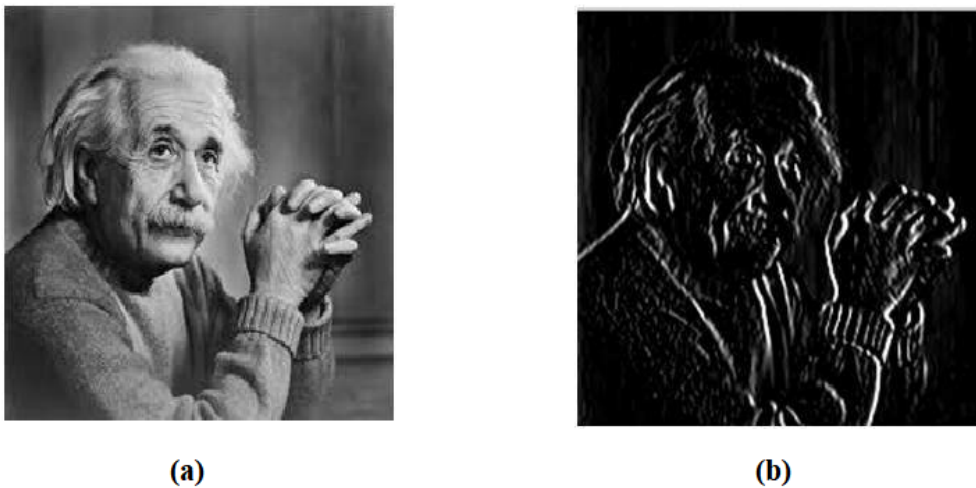
Figure 15: (a) Image I (b) Convolution of the vertical Prewitt operator and I .
