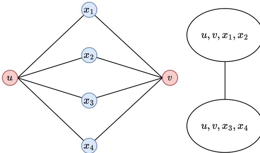
Figure 4: The graph  $K_{2,4}$  and a tree decomposition of it.
